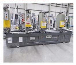
Urban welding & cleaning line: including 2 - AKS 6110/6 35/25 6 head welders & model SV800 / 2.5m, 4 head CNC corner cleaner with all transfer tables
